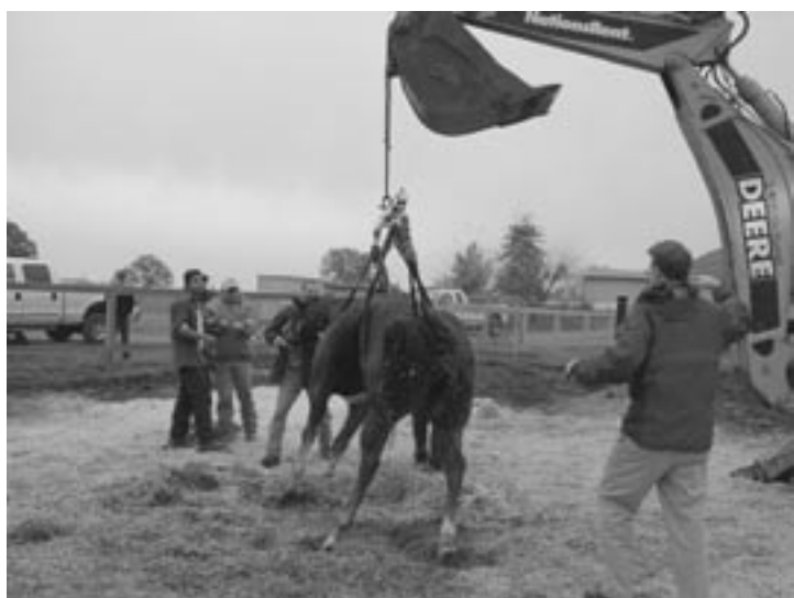
Above photo: Fitting a horse with the Large Animal Extractor. Note the counterbalance bar and two sling components.
