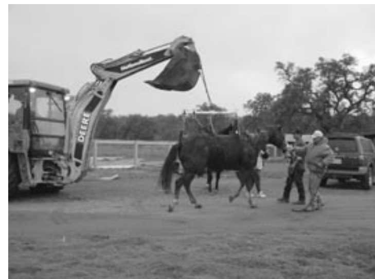
Above and below photos: When combined with construction equipment such as backhoes, forklifts, or A-frame winch-driven cranes, the extractor can easily lift these animals to the standing position.
